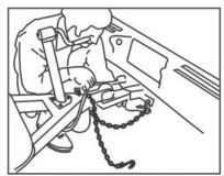
Criss-cross left chain and attach to right mounting slot in tow vehicle hitch.
