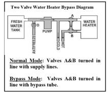
**NOTE:** In the diagram: Valve A is the black valve, valve B is the white valve. Valve D is the suction (syphon) valve that has the clear hose attached to it for siphoning in antifreeze, sanitizer or fresh water from an external container. This valve is typically located at the water pump.
