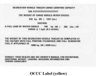
The lower portion of this label is provided voluntarily and indicates the weight value of the trailer as it was manufactured and weighed at the factory. It includes full propane tanks and full generator fuel (if so equipped).
