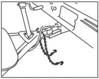
Inspect chains to determine if they are properly attached to trailer frame.
