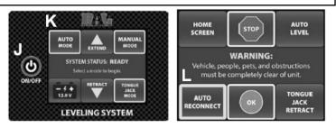
5. The system will retract all stabilizer jacks and the rear leveling jacks, then extend or retract the tongue jack until proper connection height is achieved. Display will read "Auto Reconnect in Progress". (M below)
